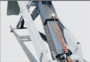
Mechanical self-lock and air-driven safety release.
