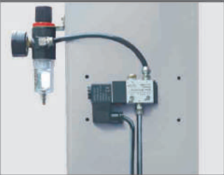
Oil-water separator and Solenoid Air Valve are installed outside the control box.
