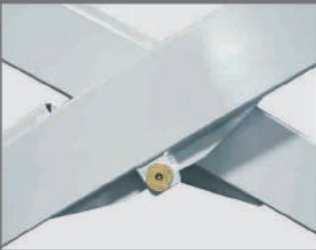
Heavy duty design, the X serial scissors lifts use 150x75mm tube to make it strong.
