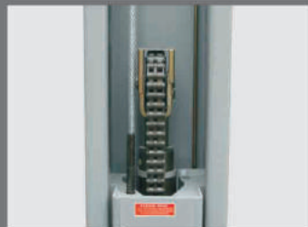
The chain overhand protection device.
