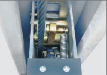
Dual safety device: In case the primary safety locks are out of operation, the lift would also be locked automatically by a second safety device.
